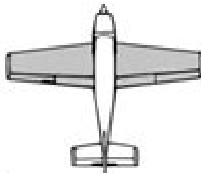
Tapered leading and trailing edges
