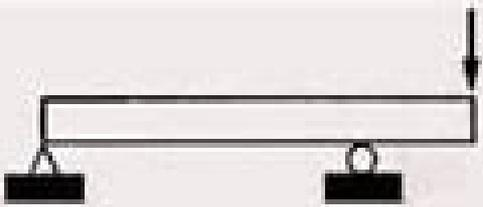
**Statically Determinate Beams**
